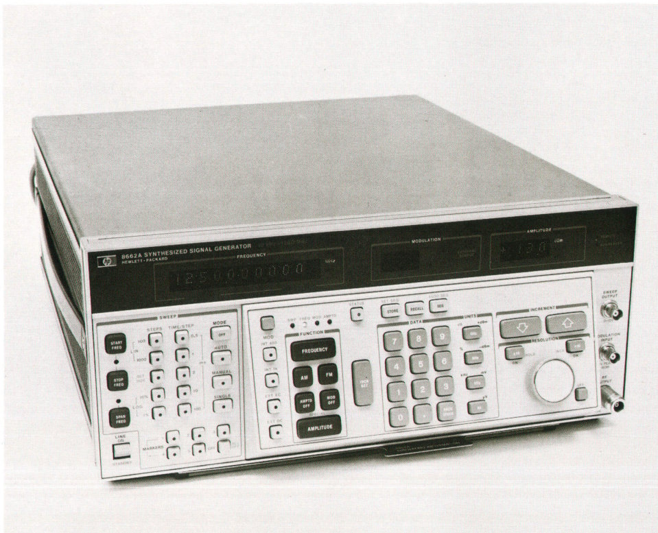
Fig. 1. Exceptionally low phase noise and spurious output make Model 8662A Synthesized Signal Generator suitable for such demanding applications as receiver adjacent channel selectivity measurements with closely spaced channels and low-noise local oscillator service. Fast frequency switching and sweep capability make the 8662A useful in frequency-agile and swept local oscillator applications. All functions are remotely programmable.
